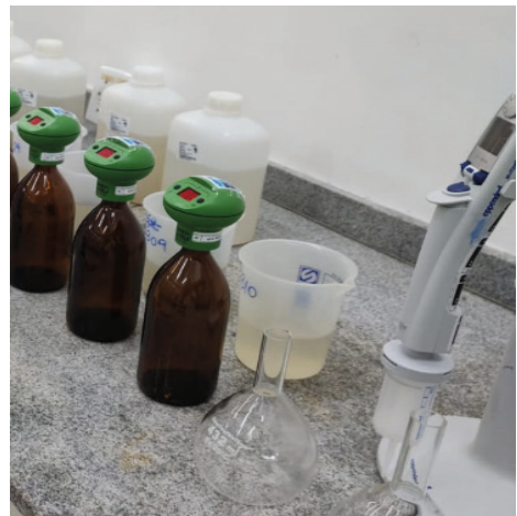
Figure 27 - BOD test preparation Source: Prepared by the author
