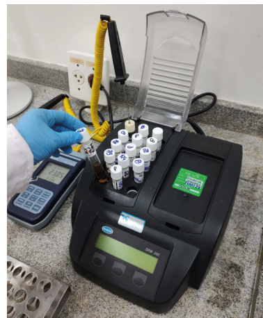
Figure 25 - COD reactor Source: Prepared by the author
