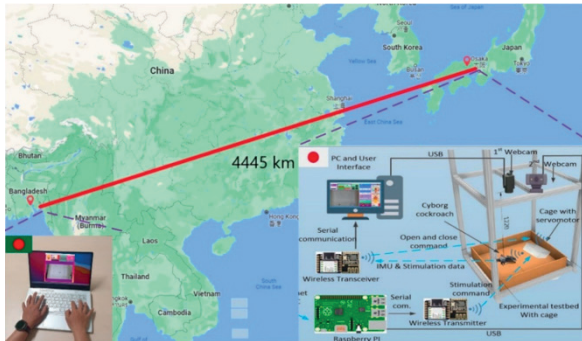
Fig. 7. Cyborg cockroaches controlled over long distances (Bangladesh and Japan) using VNC technology and RFC (Ariyanto et al., 2022).
