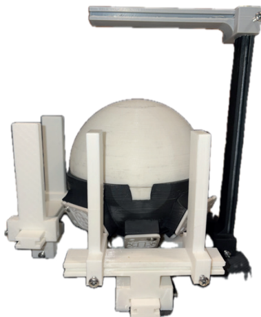
Fig. 8. Motion-tracking system 3D-printed structure.
